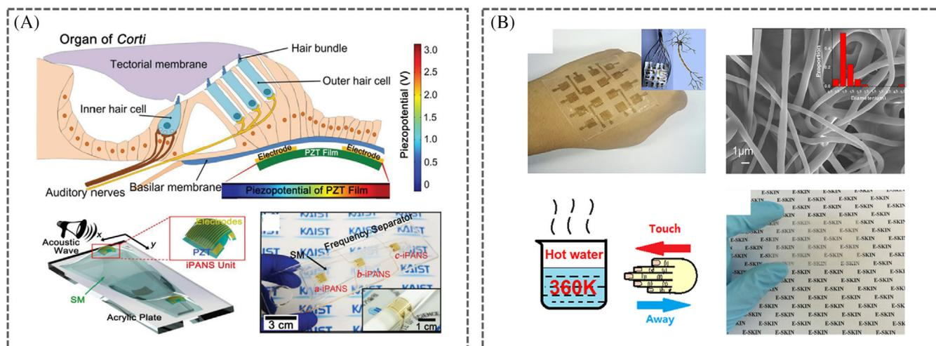
**FIGURE 6** Piezoelectric bioinspired sensors. (A) Inorganic piezoelectric acoustic nanosensors inspired by hair cells. Reproduced with permission.<sup>119</sup> Copyright 2014, WILEY-VCH. (B) Single-electrode e-skin based on piezoelectric sensor. Reproduced with permission.<sup>120</sup> Copyright 2018, American Chemical Society
