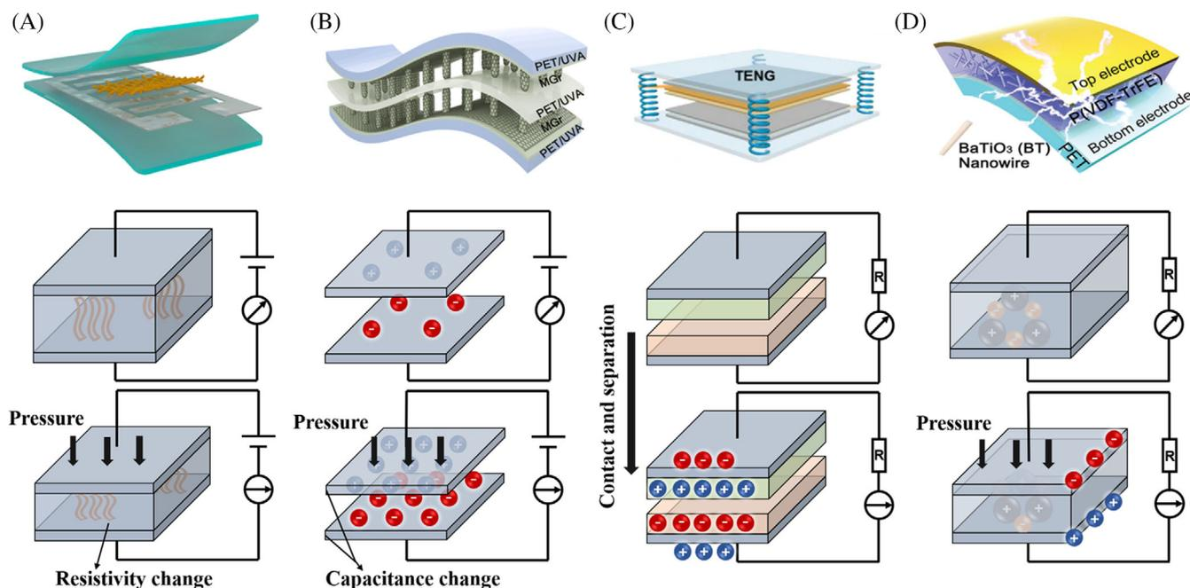
**FIGURE 2** Different working principles of bioinspired sensors. (A) Piezoresistive sensor. Reproduced with permission.<sup>100</sup> Copyright 2019 American Chemical Society. (B) Capacitive sensor. Reproduced with permission.<sup>101</sup> Copyright 2019 American Chemical Society. (C) Triboelectric sensor. Reproduced with permission.<sup>102</sup> Copyright 2020 American Chemical Society. (D) Piezoelectric sensor. Reproduced with permission.<sup>103</sup> Copyright 2018 WILEY-VCH
