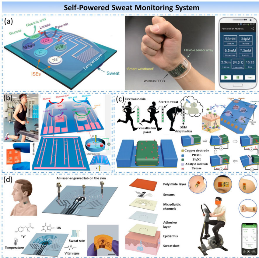
Figure 5. Self-powered sweat monitor system. (a) Multiplexed in situ perspiration analysis system based on a flexible integrated sensing array. (b) Noninvasive electronic-skin based on piezo-biosensing unit matrix. (c) Self-powered electronic-skin based on triboelectric-biosensing unit matrix. (d) Uric acid monitoring system based on an entirely laser-engraved wearable sensor.
