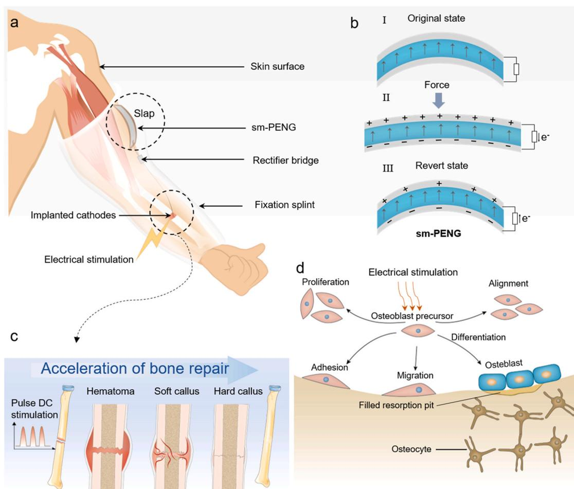
**Fig. 1.** The Schematic diagram of self-powered electrical stimulation for bone repair. a) Schematic of the integrated self-powered pulsed-DC device based on sm-PENG and fracture fixation splint for bone repair in vivo. b) Working principle of the PVDF piezoelectric layer. c) Electrical stimulation accelerates bone repair. d) Effect of electrical stimulation on osteoblast precursor behavior.
