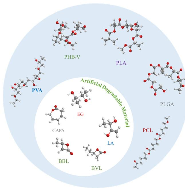
**FIGURE 5** Artificial degradable material used in TENG and its monomer; BBL,  $\beta$ -butyrolactone; BVL,  $\beta$ -valerolactone; CAPA, caprolactone; EG, ethylene glycol; LA, lactic acid; PCL, polycaprolactone; PHB/V, poly(1-hydroxybutyrate valerate); PLA, polylactic acid; PLGA, poly(lactic-co-glycolic acid); PVA, polyvinyl alcohol
