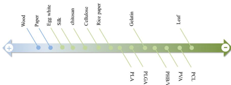
**FIGURE 9** Triboelectric series<sup>12,13,16,96,97</sup> of degradable materials based on their ability to lose or gain electrons. The reference material is PDMS
