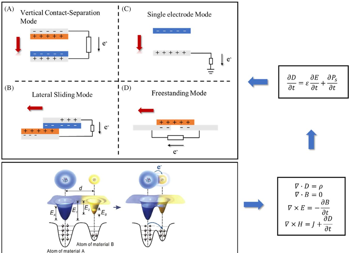
**FIGURE 2** (A-D) Schematic diagram of structures and mechanisms of TENG.<sup>31,32,35,36</sup> (e) CE mechanism explained by electron cloud-potential well model at high temperatures<sup>37</sup>
