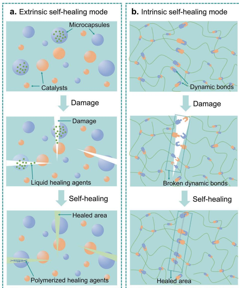
**Figure 2.** Extrinsic self-healing mode (a) and intrinsic self-healing mode (b).
