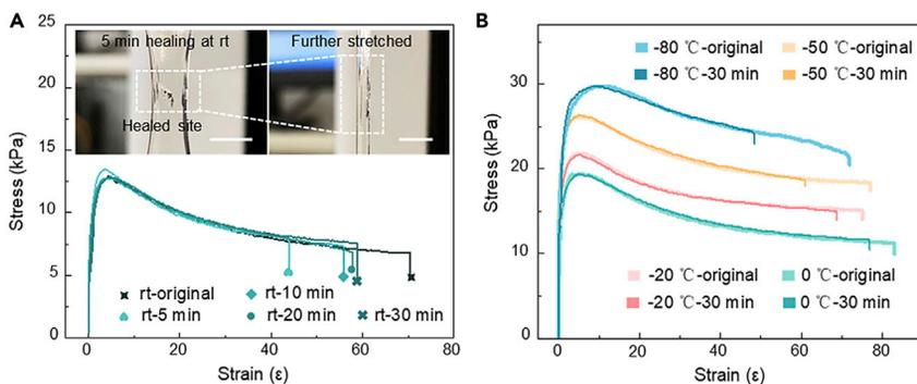
**Figure 4. The tensile stress–strain curves of the ionic hydrogel at the original state and after 30 min healing in various temperatures**
