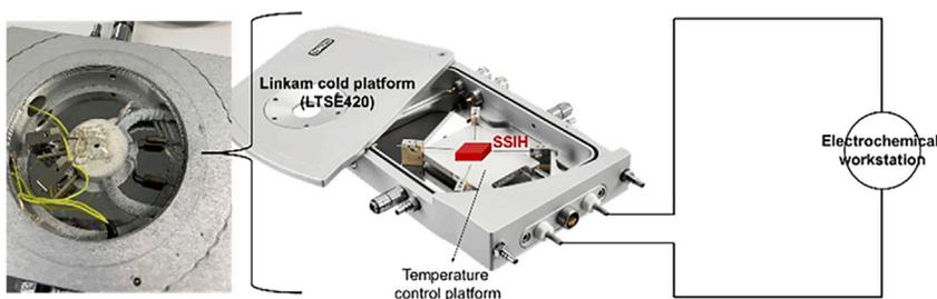
**Figure 3.** The electrochemical performance of ionic hydrogels tested with LTSE420/CHI 660E
