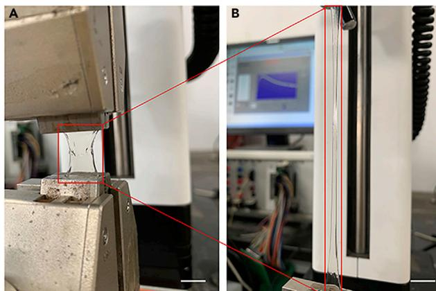
**Figure 2. The stretchability was tested with ESM301/Mark-10 system**
