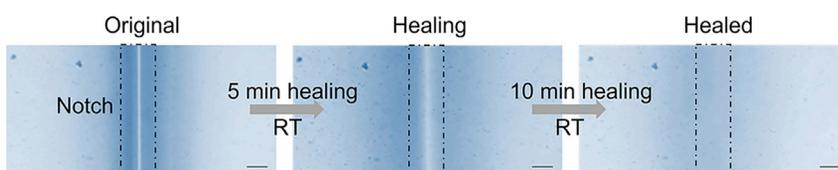
**Figure 5. The self-healing process of the damaged ionic hydrogel was observed through the optical microscope** Scale bar: 1 mm. Reproduced with permission (Wang et al.).<sup>1</sup>
