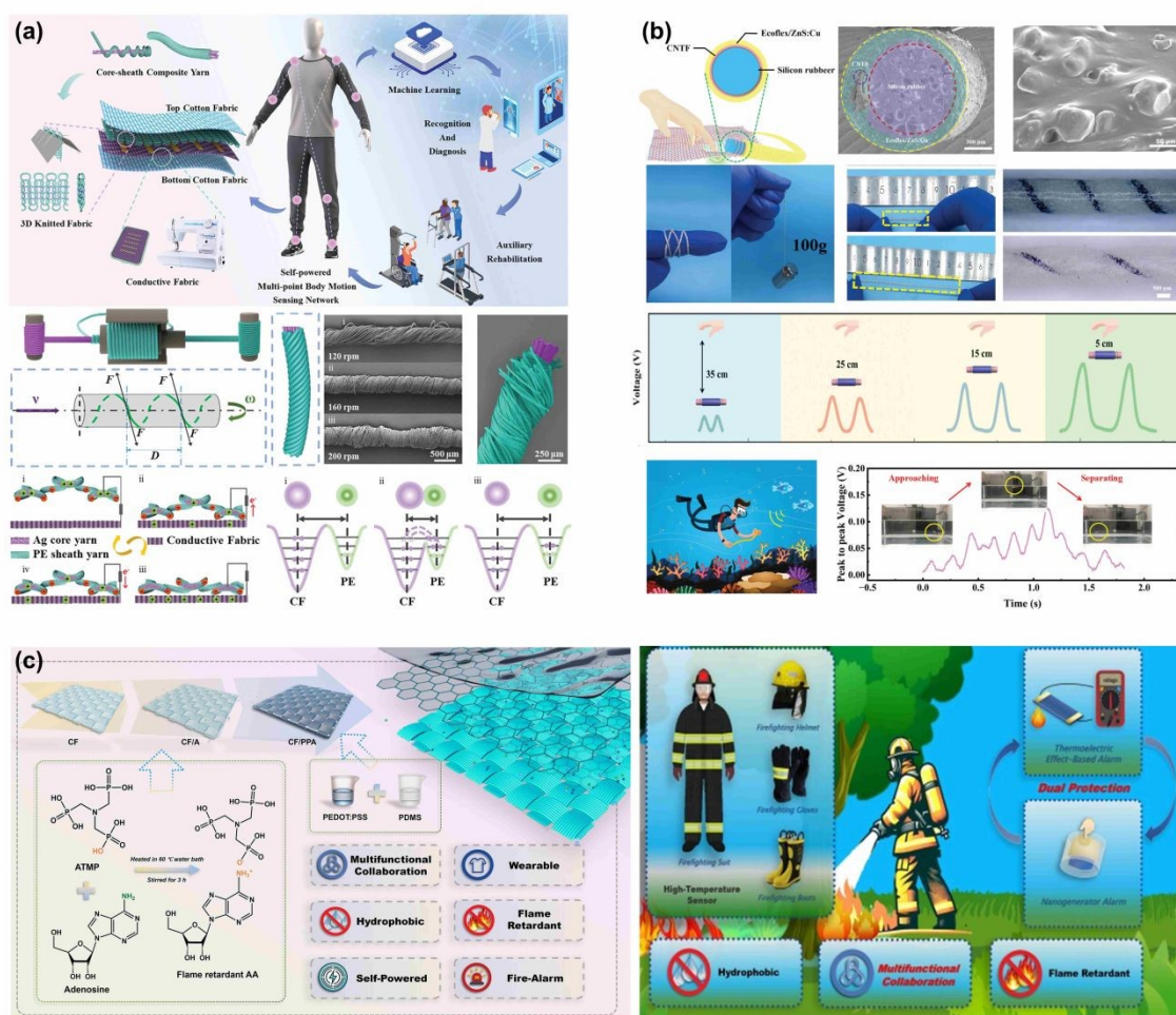
Fig. 8 Smart fabric. (a)Structural design of textile-based SMN and schematic diagram of a highly integrated gait recognition system. Schematic diagram of the manufacturing process and parameters of Ag-PE core-sheath composite yarn. Atomic-scale-electron-cloud potential-well model to describe the contact electrification between conductive fabric and PE sheath yarn. Reproduced with permission from ref. 154 . Copyright 2023 Wiley-VCH GmbH. (b)Schematic diagram and SEM image of MLTENG principle. Photos of stretchable MLTENG and their corresponding optical images and dynamic loading structure diagrams. Output voltage of MLTENG at different distances and its application and transmission in water. Reproduced with permission from ref. 155 . Copyright 2024 The Author(s). Advanced Science published by VCH GmbH. (c)Illustration of the synthetic route of conductive fabric/Polyphthalamide. Application of Fire Alarm System Based on Thermoelectric Effect and TENG. Reproduced with permission from ref. 156 . Copyright 2024 Elsevier B.V. All rights are reserved, including those for text and data mining, AI training, and similar technologies.
