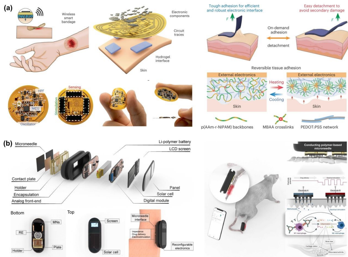
Fig. 12 Precision treatment. (a) Schematic diagram and exploded view of the wireless smart bandage including FPCB and tissue-interfacing conducting adhesive hydrogel. The schematic diagram for the hydrogel interface in the smart bandage. Schematic diagram illustrating microscopic structural changes during LCST phase transition. Reproduced with permission from ref. 184 . Copyright 2022, The Author(s), under exclusive licence to Springer Nature America, Inc. (b) Mechanism of drug and electrical stimulation synergistic therapy using an integrated smart device. Rodent models are used to collect clinical parameters to train and validate machine learning models and to evaluate the outcomes of synergistic treatments. Reproduced with permission from ref. 185 . Copyright 2024, The American Association for the Advancement of Science.
