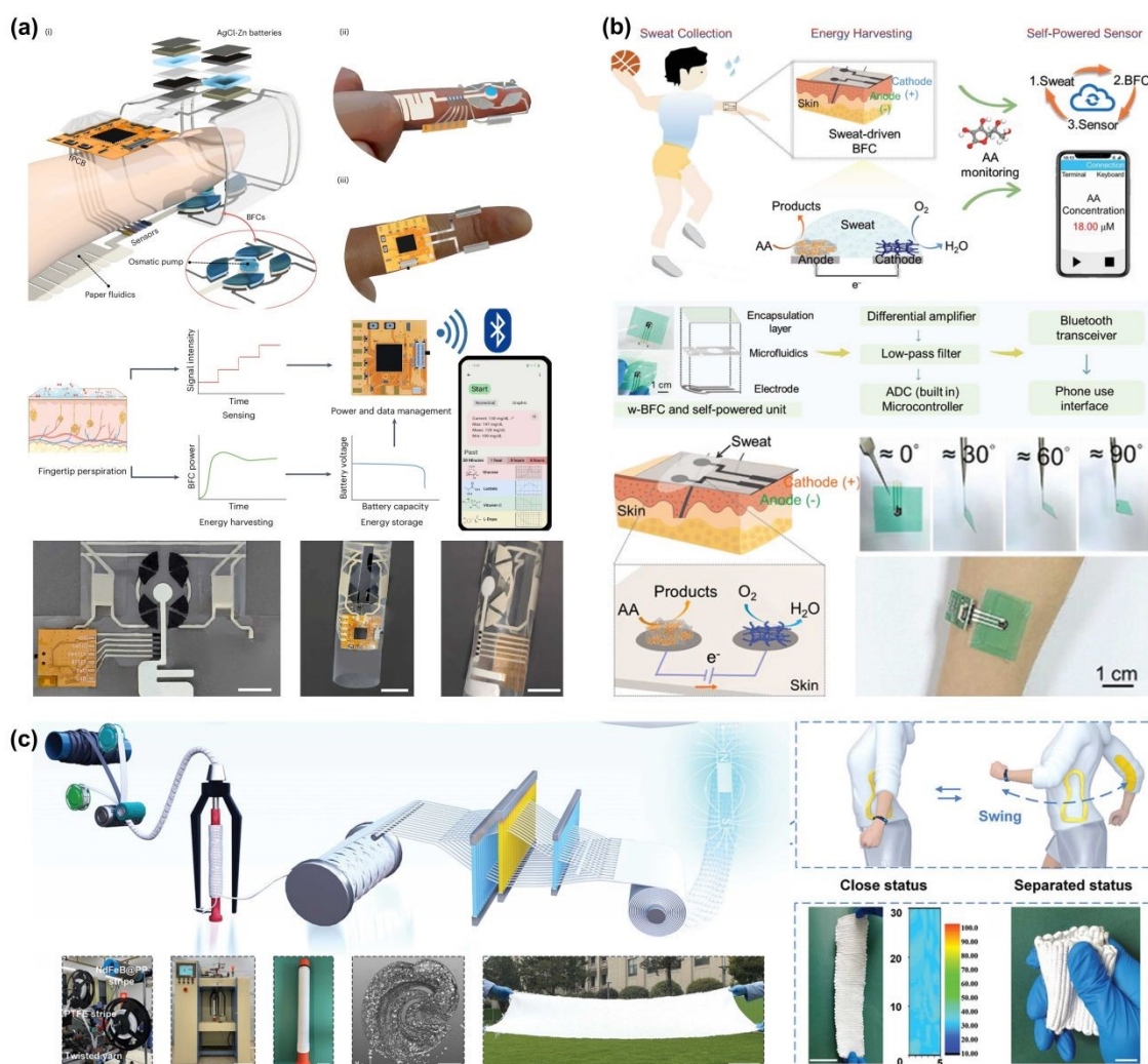
Fig. 6 The application cases of BFCs and magnetoelectric effect. (a) Fingertip-wearable microgrid system schematic, working principle schematic, and optical image. Reproduced with permission from ref. 51 . Copyright 2024, The Author(s), under exclusive license to Springer Nature Limited. (b) Schematic illustration of the metal hydrogel-based integrated w-BFC for sweat collection, energy harvesting, and self-powered sensor. Reproduced with permission from ref. 52 . Copyright 2024 Wiley-VCH GmbH. (c) The process of preparing magnetic fabric. Microcomputerized tomography images of NdFeB magnetic yarn. A piece of 1 × 3 m 2 plain weave fabric formed by industrial weaving
