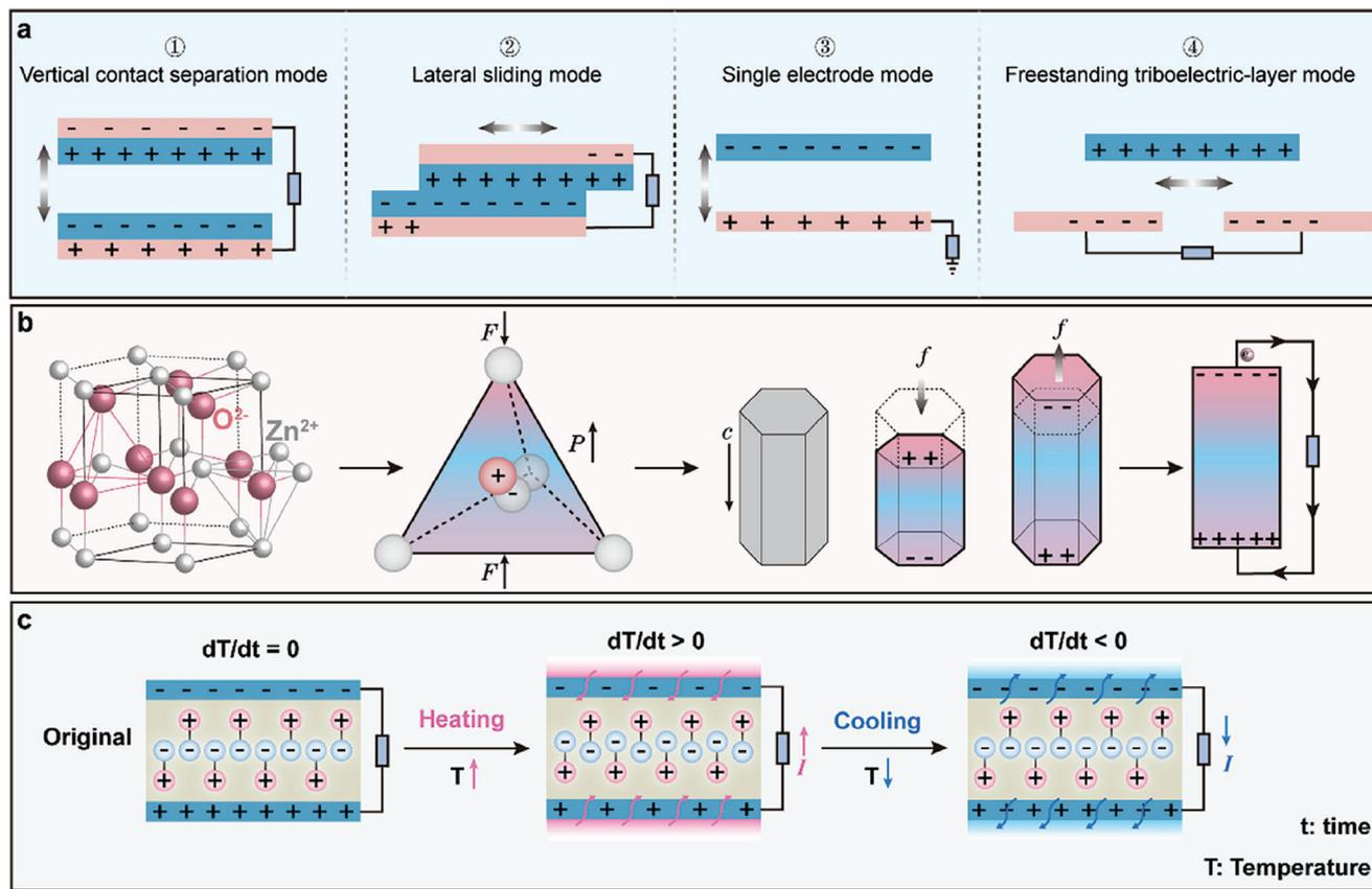
**Figure 3.** The classification and working principles of NGs. a) Four fundamental working modes of the TENG. b) Working modes of the PENG based on the ZnO nanowire. c) Working principles of the PyENG.
