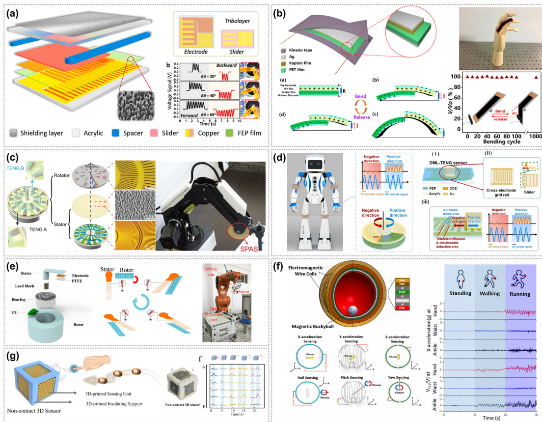
Fig. 7. Nanogenerator-based vector motion sensors. (a) Joint motion triboelectric quantification sensor (jmTQS) to detect the degree and speed of flexion/extension movements in fingers [122]. Copyright (2023) by Elsevier. (b) TENG-based stretchable sensor to detect motion and angle information [123]. Copyright (2018) by MDPI. (c) Rotating grating-structured self-powered angle sensor based on TENG [124]. Copyright (2023) by John Wiley and Sons. (d) Vector motion sensor based on dual-mode TENG to judge movement direction and angle [121]. Copyright (2023) by Elsevier. (e) TENG-based non-contact sensor to detect rotational movement [125]. Copyright (2020) by MDPI. (f) 3D activity inertial sensor (3DAIS) based on electromagnetic, piezoelectric, and triboelectric technologies [126]. Copyright (2023) by Elsevier. (g) CNF/MXene-based deep-trap hierarchical architecture for high-performance TENG [127]. Copyright (2023) by Elsevier. (For interpretation of the references to color in this figure legend, the reader is referred to the web version of this article.)
