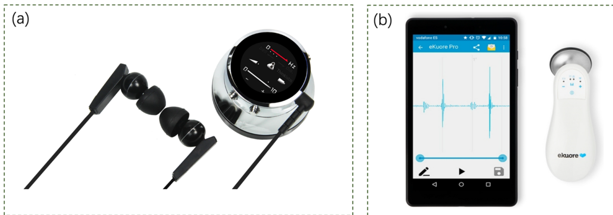
Figure 2. Examples of electronic stethoscopes. (a) The Thinklabs One [37]. (b) The eKuore stethoscope [37].
